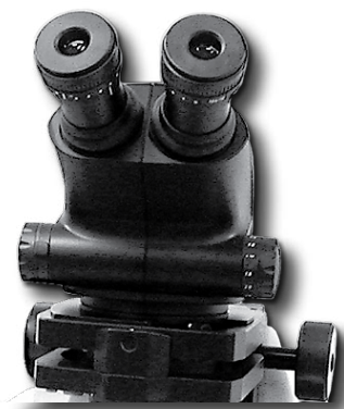
Stereomicroscope with Scan and Tilt Range: 10.08X to 64X with standard 16X eyepieces
