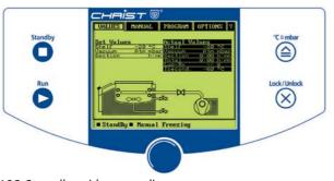
LSC-Controller with system diagram
